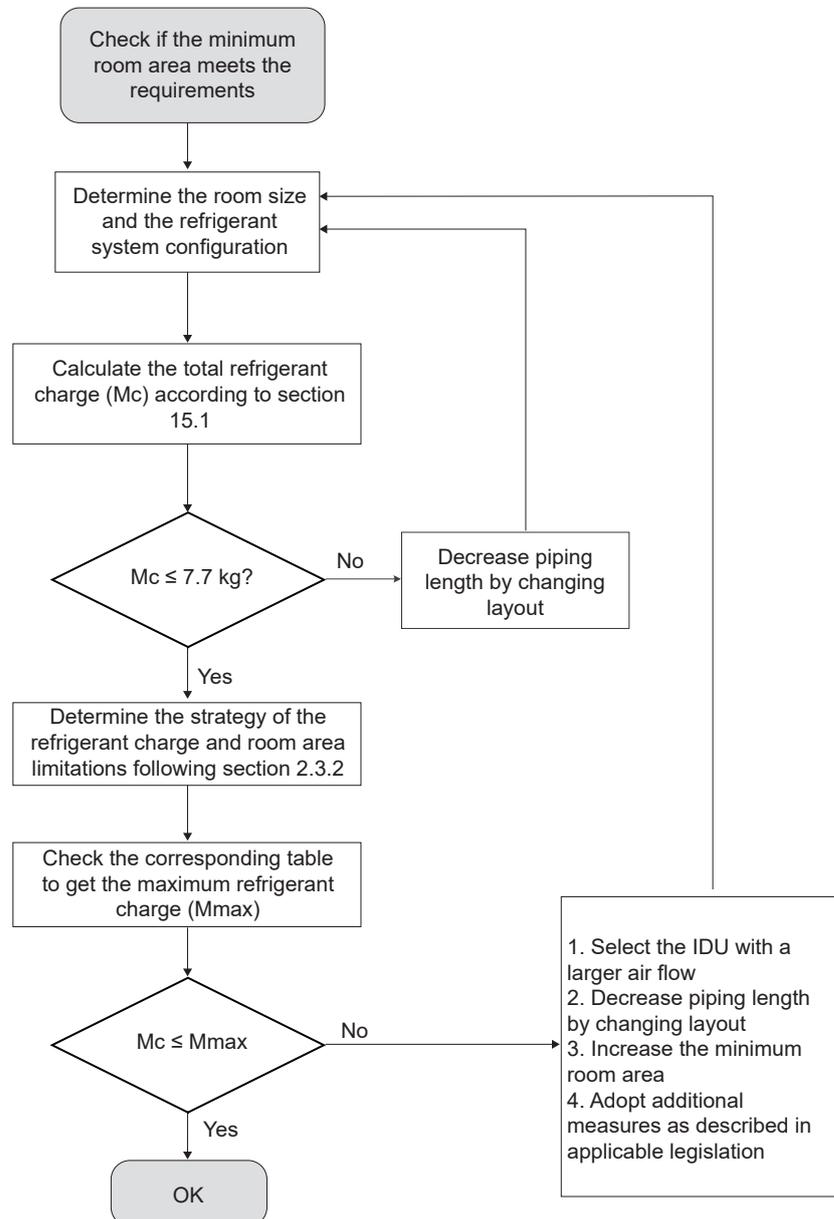
In addition, the maximum refrigerant charge is also related to the installation height of the DHW kit and hydraulic module of the IDU. The correspondence of the maximum refrigerant charge with the minimum room area ( $A_{min}$ ) is shown in Figure 1 and Table 1. And different values are used for different indoor installation heights:
