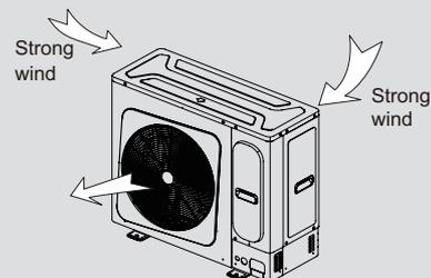
It is recommended that the fan direction of the discharge port be set at right angle to the wind direction.
