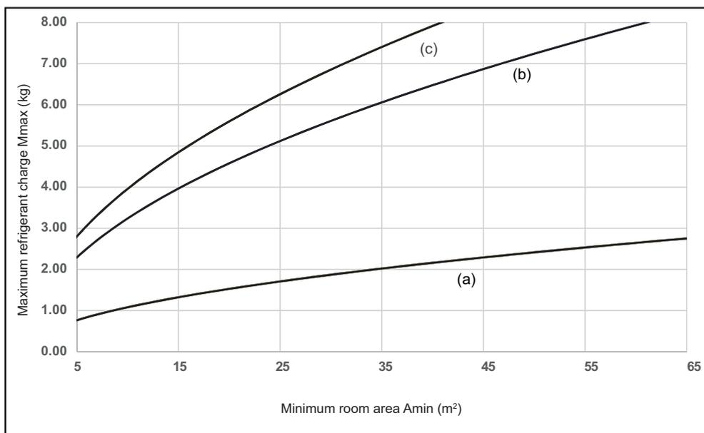
Curve (a) is the refrigerant charge limit for the IDU installation height  $h \geq 0.6$  m
