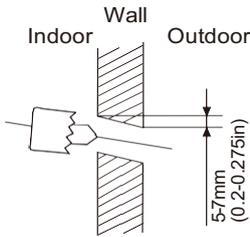
**NOTE:** When the gas side connective pipe is  $\Phi 16\text{mm}$ (5/8in) or more, the wall hole should be 90mm(3.54in).
