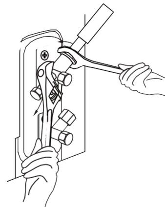
5. While firmly gripping the body of the valve, use a torque wrench to tighten the flare nut according to the correct torque values.
