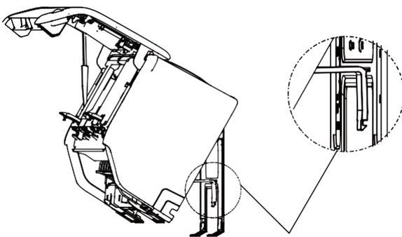
Use the holder at the back of the unit against on the mounting plate to prop up the unit
