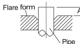
6. Place flaring tool onto the form.
