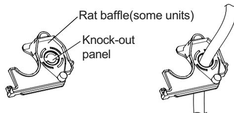
**NOTE:** If the size of the cable is too big, remove the middle small plastic knock-out panel to create a slot through which the cable can exit. If you want to remove the chassis or drain hose, please remove the rat baffle first.
