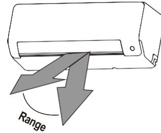
**NOTE:** Do not move louver by hand. This will cause the louver to become out of sync. If this occurs, turn off the unit and unplug it for a few seconds, then restart the unit. This will reset the louver.
