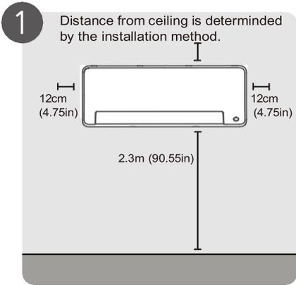
**1** Distance from ceiling is determined by the installation method.
